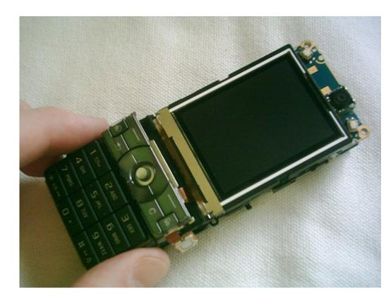
The screen assembly is held on by two clips at each side of the phone, indicated below. Unclip them to remove the screen assembly
