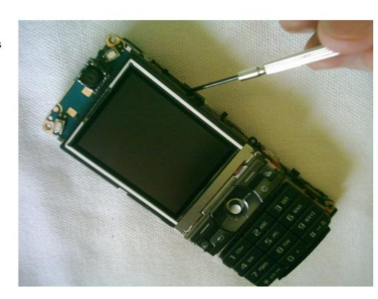
Unclip the ribbon which hold the screen assembly to the circuit board of the phone. It attaches like a plug and socket
