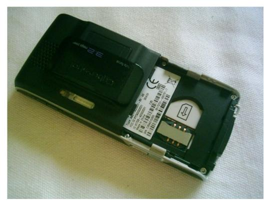
Lift the antenna cover away from the phone. It unclips at the top of the phone and needs a little force to remove
