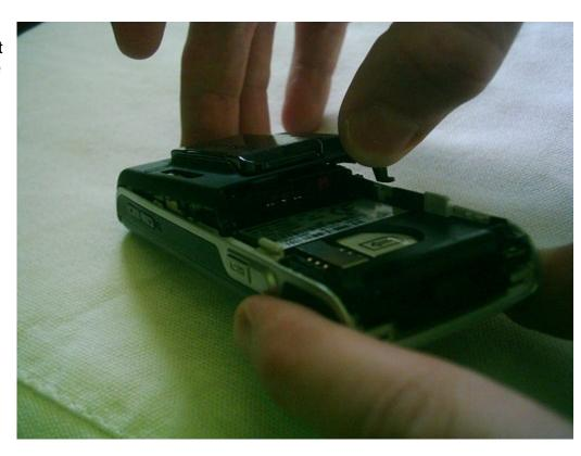
Remove the two torx 6 screws at the top of the phone which are revealed after removing the antenna cover
